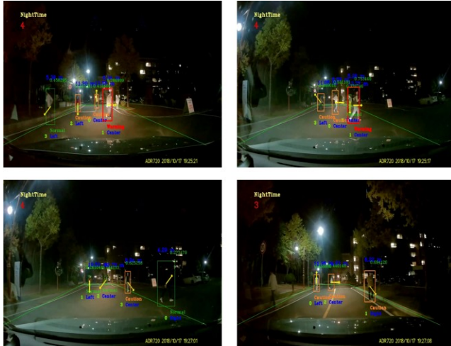
Figure 2 Sample RPC prediction results using the proposed method. Red box, orange box, green box means ‘Warning’, ‘Caution’ and ‘Normal’ respectively. The arrows represent the orientation of pedestrian and numbers represent the distance pedestrians from the camera.
